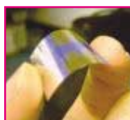
A FET (field effect transistor) on a flexible substrate
